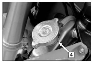
A mixture of 50% antifreeze liquid and 50% destilled water is used as coolant. However, the antifreeze protection must be at least -25 $^{\circ}$  C (-13 $^{\circ}$  F). This mixture offers antifreeze protection but also good corrosion protection and should therefore not be replaced by pure water.
